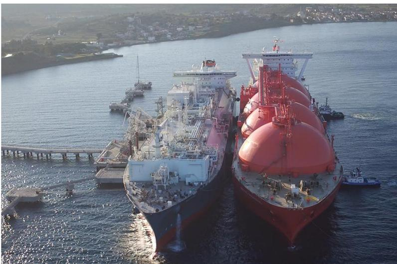
Example of a floating storage and regasification unit and liquid natural gas ship. Image: Höegh LNG.
